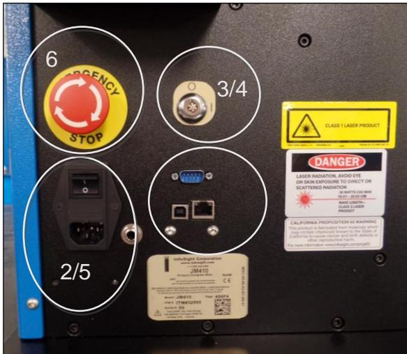
USB & Ethernet ports exist under the RS 232 port (1, above). Refer to the Communications Section of this manual for instructions on installing the required drivers.
